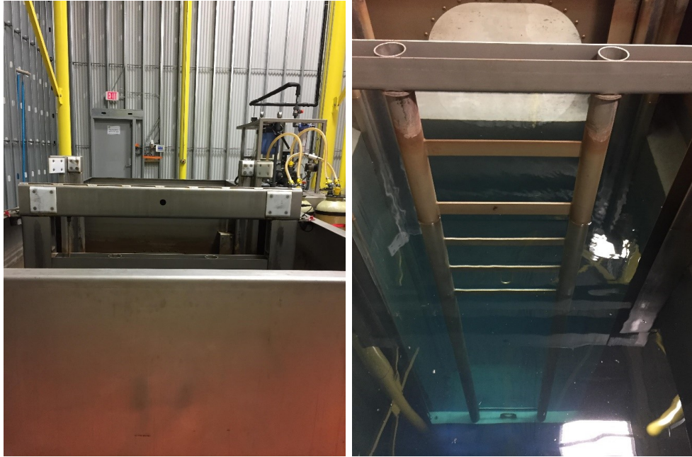
Figure 2.3 Storage pool of irradiation source. Photo were taken in an USDA/APHIS certified phytosanitary treatment facility located in Gulfport, MS (Gateway America).
